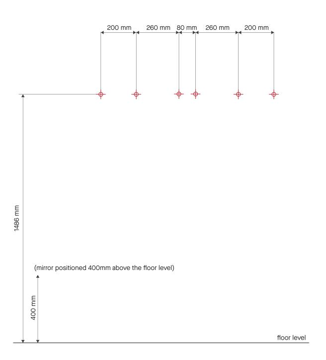
place the mirrors on the washers in the 'open' position once all pieces are placed on the wall slide the left and right mirror toward the central mirror leave a 5cm gap between the big mirrors in order to show the black mirror
