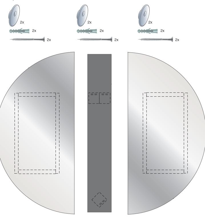
mark the suspension point on your wall drill holes and place the plugs, washers and screws
