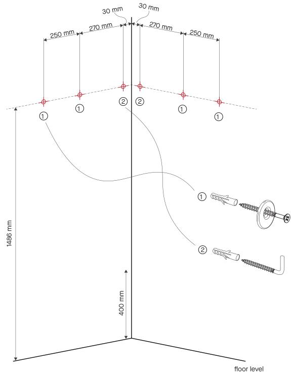
(mirror positioned 400mm above the floor level)
