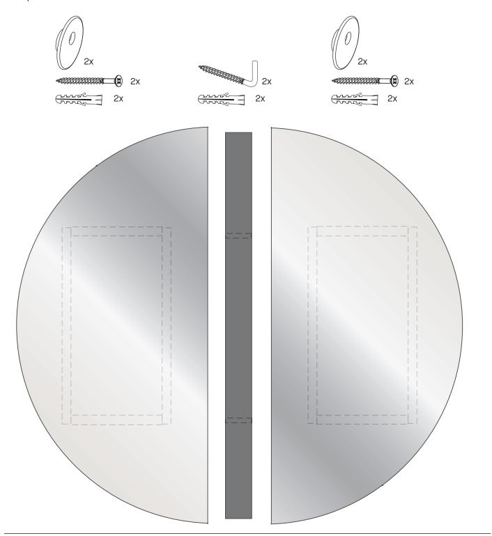
mark the suspension point on your wall drill holes and place the plugs, washers and screws or plugs and hooks
