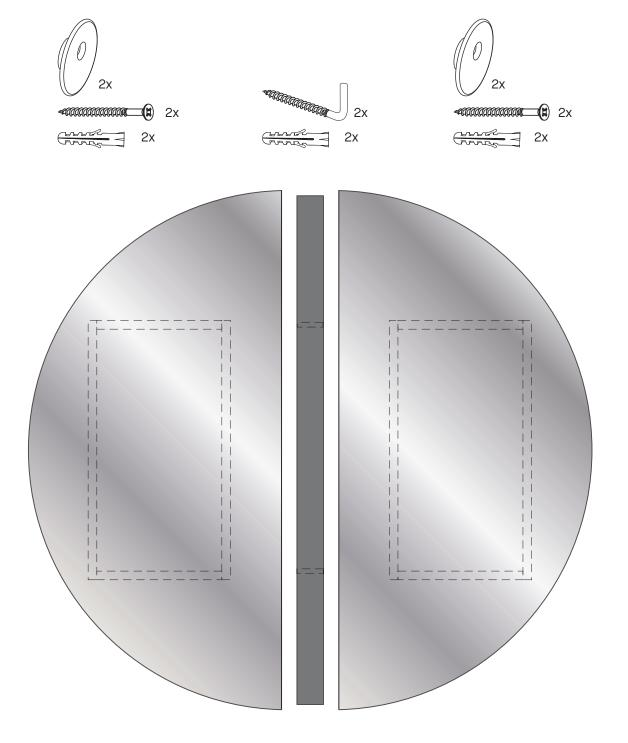
mark the suspension point on your wall drill holes and place the plugs, washers and screws or plugs and hooks
