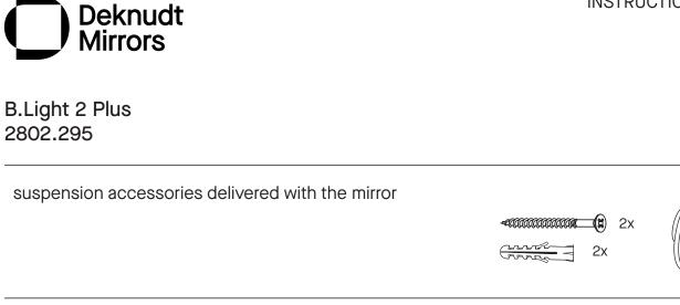
Mark the suspension point on your wall drill holes and place the plugs, washers and screws. The washers allow you to slightly adjust the level of the mirror.
