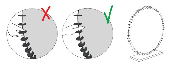
Do not lift the mirror at the frame as the metal lamellae may bend out of shape.
